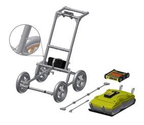
Attach the GPR Sensor to the Cart using the Sensor Support Straps. Ensure the Sensor is oriented the correct way with the connections toward the back of the Cart. Using the Sensor Support Straps, adjust the height of the Sensor so it is 1-2 cm ( $\frac{1}{2} - \frac{3}{4}$  inch) above the ground. The best way to get a uniform Sensor height is to place a couple of sheets of thick cardboard, particle board or Styrofoam under the sensor before securing the Sensor Support Straps.
