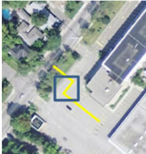
The yellow line shows the anticipated location of the gas pipe.
